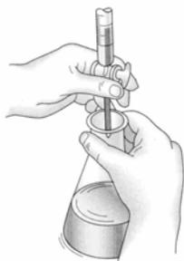
Look at the position of the piston. Is the buret full? If not, press **Fill**. When the buret is full, it will automatically switch back into delivery mode.
